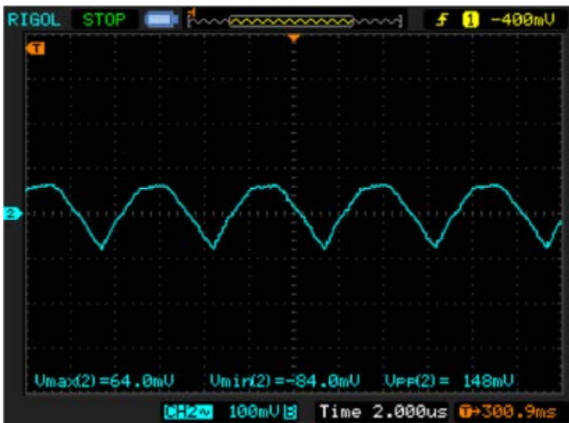
Figure 3. Output ripple at 800mA load, 12V OUT .
