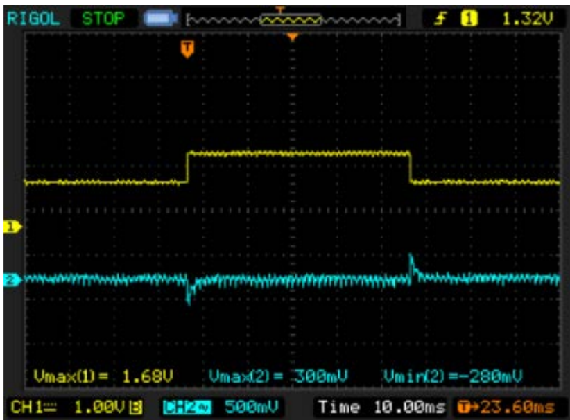
Figure 5. Transient response when load steps from 960mA to 1600mA.
