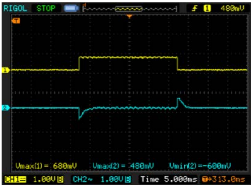
Figure 4. Transient response when load steps from 5mA to 640mA.
